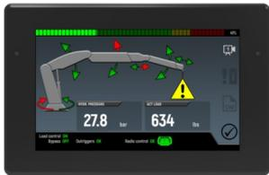
Vscale E3 operator terminal with two CAN interfaces (Source: Wika)
