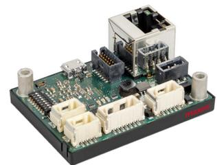
The Micromacs6 from Maxon Motor with two CAN interfaces (Source: Maxon Motor)
