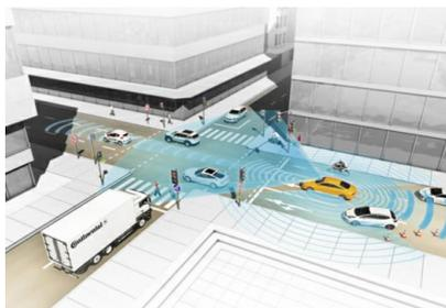
*Automated driving requires detection of the environment by means of sensors; the drive commands at the end of the process are transmitted via the CAN-based in-vehicle networks*
