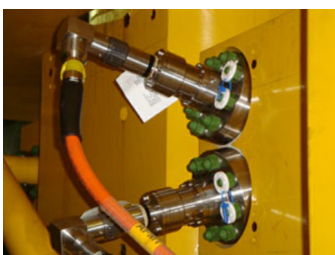
TPT SIIS-L2 pressure and temperature transmitter by Transcontrol
