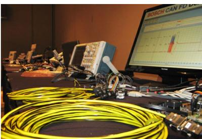
*The CAN FD demonstrator runs at an arbitration data-rate of 1 Mbit/s and 10 Mbit/s during the dataphase with a total network length of 40 m using off-the-shelf CAN transceiver chips*
