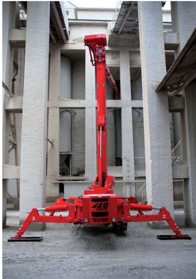
Figure 1: The LEO platform with stabilizer
