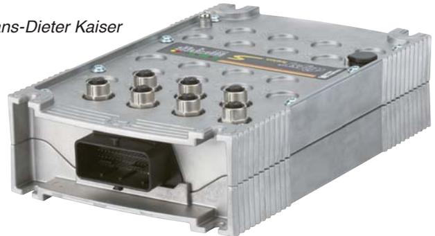
Figure 2: Safety controller digsy fusion S
