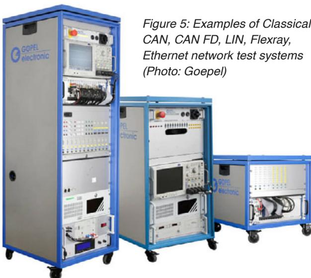
Figure 5: Examples of Classical CAN, CAN FD, LIN, Flexray, Ethernet network test systems (Photo: Goepel)
