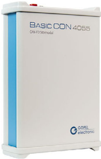
Figure 3: Basic CON 4055 stress and trigger module (Photo: Goepel)
