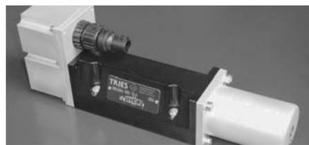
The 391 series of 4/3-directional control valves by Tries are pilot-operated restrictor valves, which work according to the pressure dividing principle. The pilot actuation is realized by a linear motor. The housing contains electronics for activation and analysis and may be turned by 90°. The
