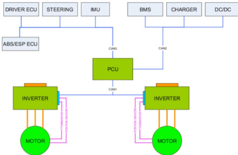
Figure 2: Conceptual schematic of separate CAN communication networks within a distributed powertrain system (Source: Elaphe)
