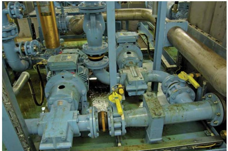
Figure 2: Hydraulic pumping unit in a steel mill
