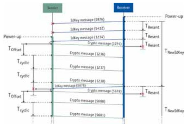
Figure 1: Message transmission and timing of encrypted communication
