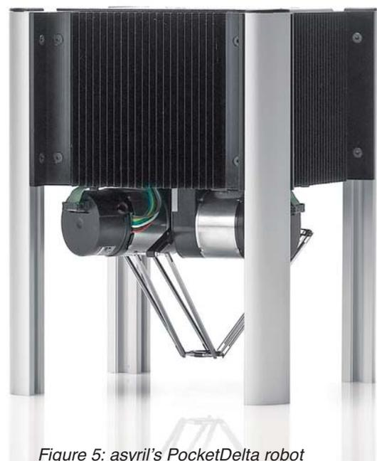
Figure 5: asyriil's PocketDelta robot
