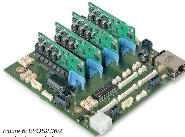
Figure 6: EPOS2 36/2 positioning controllers with motherboard
