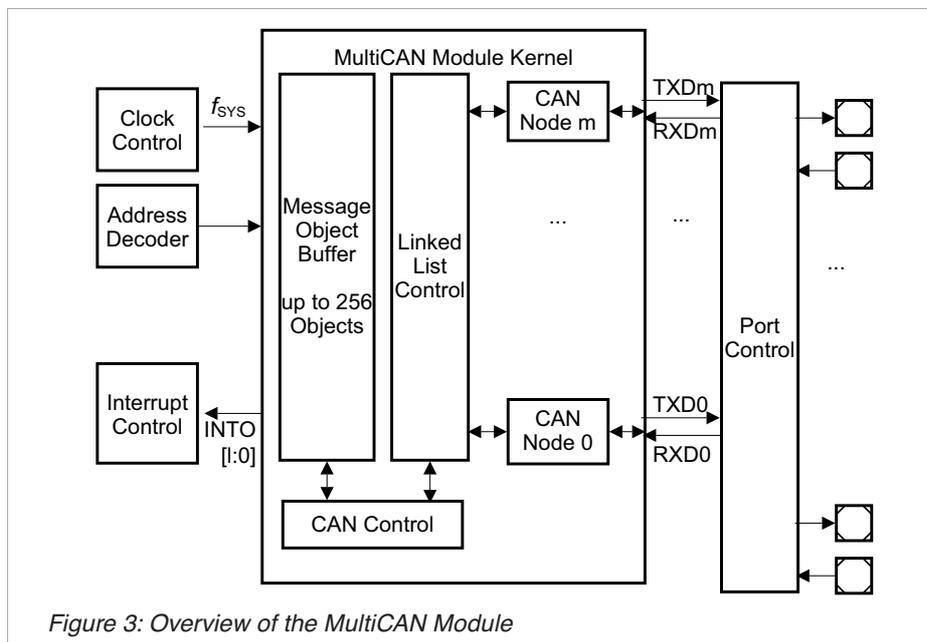
Figure 3: Overview of the MultiCAN Module
