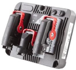
Figure 3: The GL84 is for centralized control system architecture where one commander/central unit controls multiple responders. It has a whopping 27 GND pins for sensors and actuators and CAN1 is also routed to M12 connectors for wiring. (Source: Epec)
