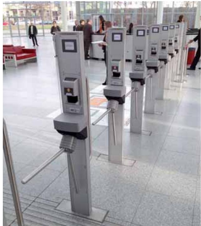
Figure 2: Typical turnstile applications at Venice's Vaporetto stations (Venice) and on the Vienna fair-ground controlling the access and counting the number of people passing through (Source: Axxess)
