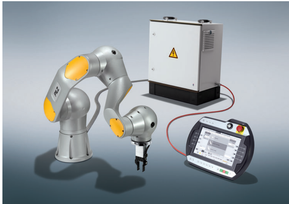
Figure 1: The shown modules are designed for service robot applications in industrial environments (Photo: Pilz)
