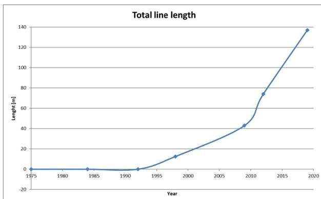
Figure 1: Total network length in Golf cars, which needs to be reduced in future vehicles to save weight (Source: VW)
