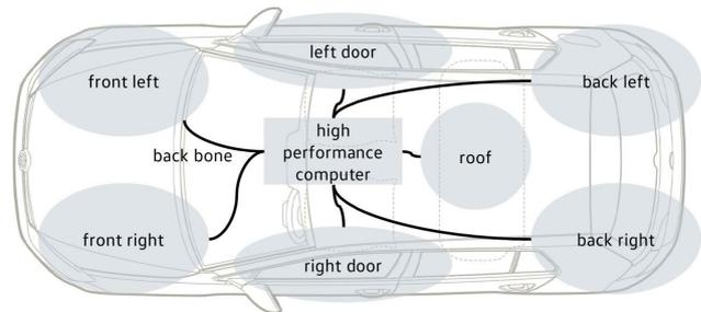
Figure 2: Zone networking architecture example (Source: VW)
