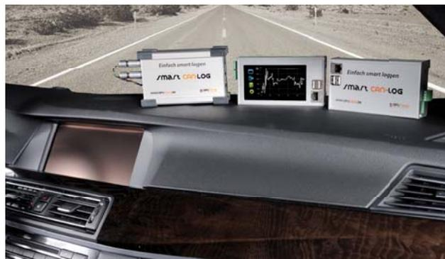
Figure 2: Different housing options of the smartCANLog
