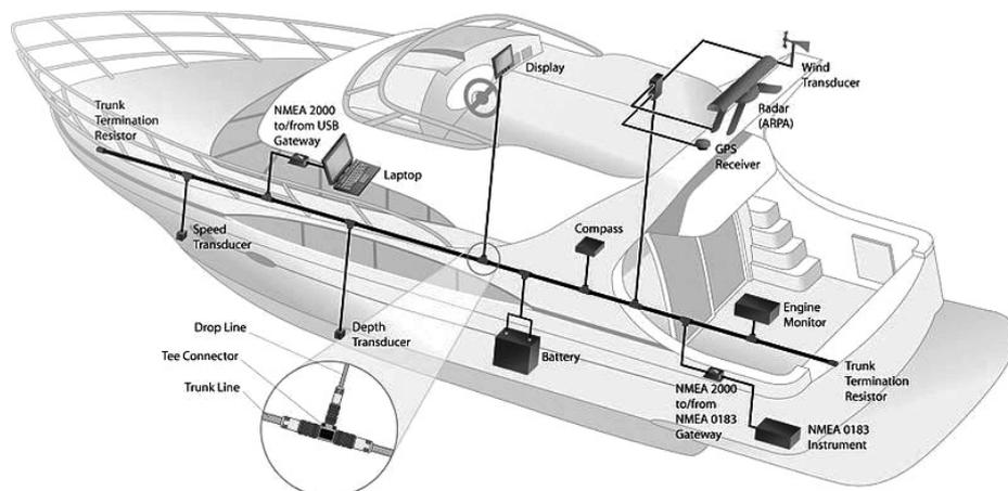
Figure 2: A typical NMEA 2000 installation (Source: NMEA)
