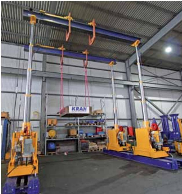
Figure 5: Lifting device for heavy loads
