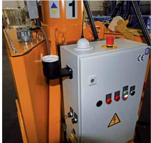
Figure 7: Electric control cabinet for a leg of the lifting facility
