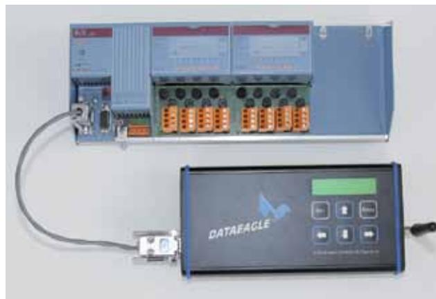
Figure 2: DE 6000 with a controller of Bernecker + Rainer coupled to a S7 PLC
