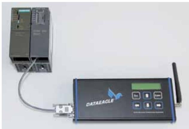
Figure 1: DE 6000 used with a CAN module by Helmholz on a S7 PLC
