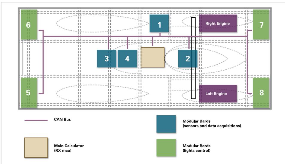
Figure 3: CAN network structure in the vehicle
