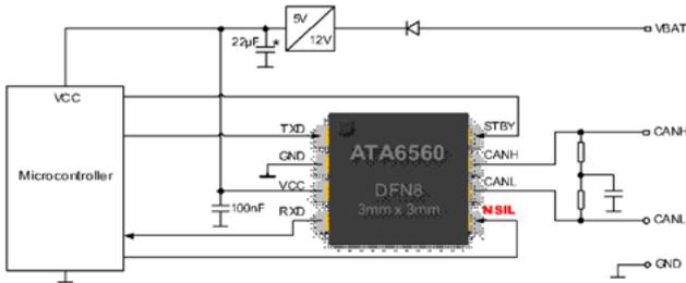
Figure 2: Typical application circuitry using the ATA6560 (Source: Atmel)
