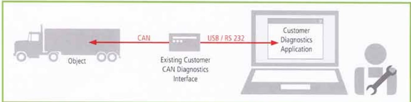
CAN data is read via cable connection – remote diagnosis is not possible.
