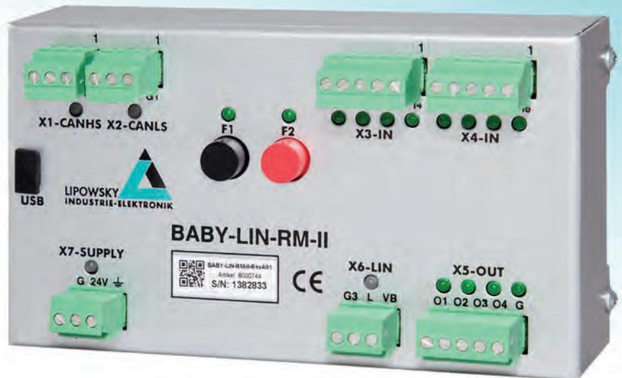
LIN & CAN Bus simulation with digital I/O
