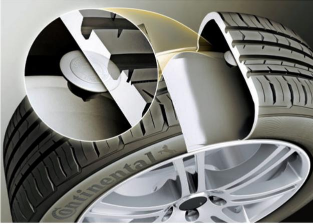
Figure 1: Being integrated directly into the inner liner of the tire means that the eTIS sensor offers data to the CAN-based receiver unit that can be forwarded to interested ECUs (Photo: Continental)
