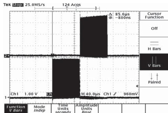
Figure 2: Delay introduced by a Switch (best case)
