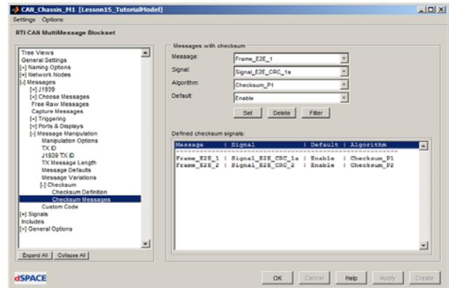
Figure 2: Pre configuration of CRC algorithms with the RTI CAN Multi Message Blockset
