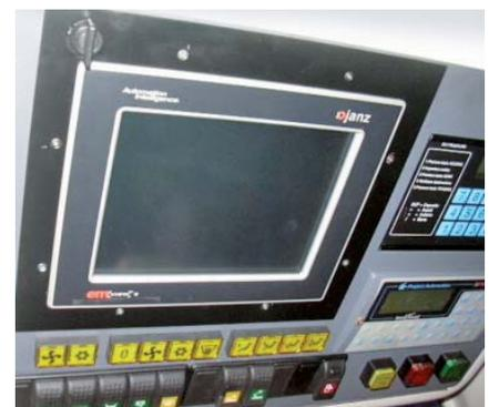
Figure 2: The EmView panel-PC installed in driver's cabin
