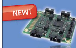
PCI/104-Express interface board with up to 4 CAN channels, low-speed CAN and LIN.
