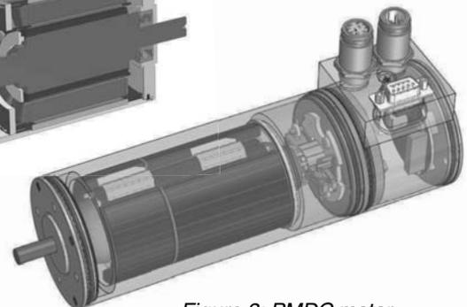
Figure 3: PMDC motor (PC 6355) with integrated CAN interface
