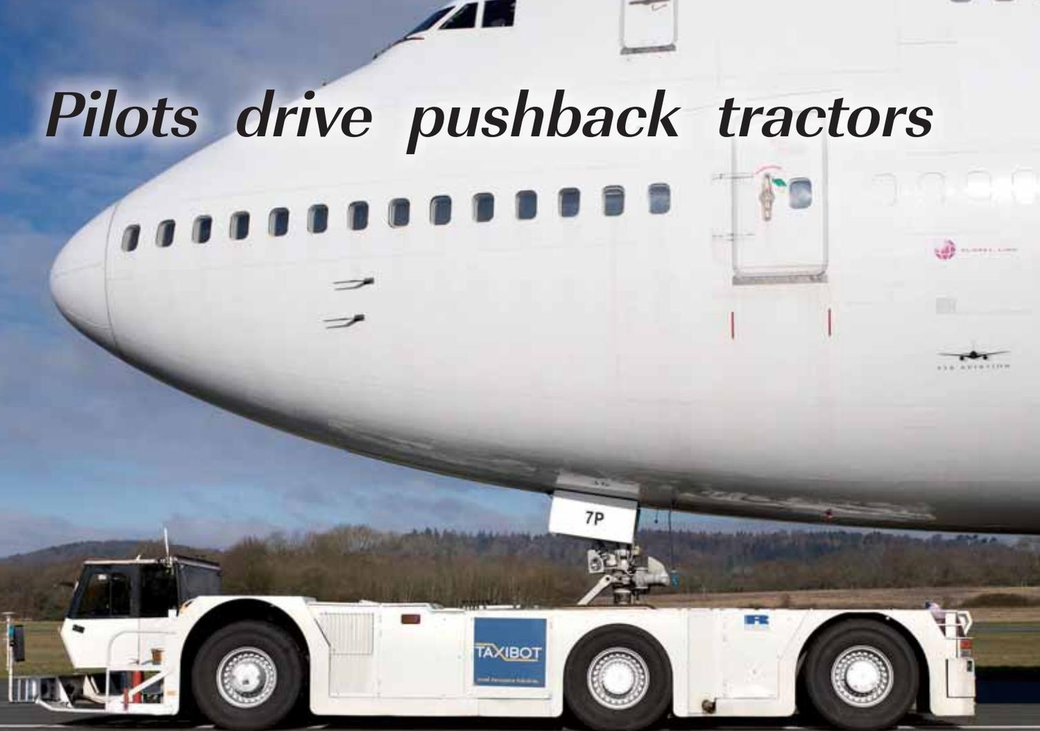
*Before take off, airplanes have to be towed. Pilot-controlled Taxibots can do that without running engines, saving fuel. The tractors are based on CAN-connected position sensors and control systems.*
