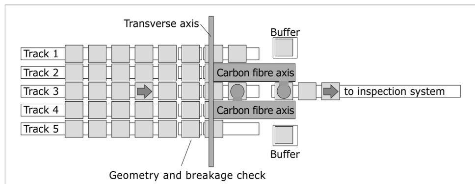
Figure 1: Wafer transfer system with incoming and outgoing wafers
