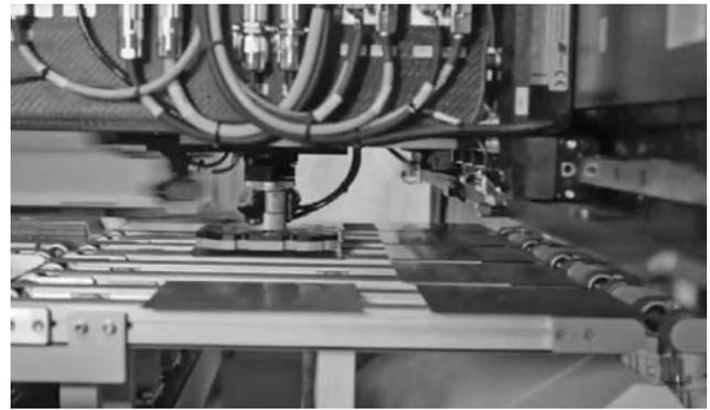
Figure 3: Wafer pick-up unit
